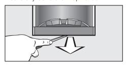
■ Carefully remove the drip tray using a screwdriver if necessary.
